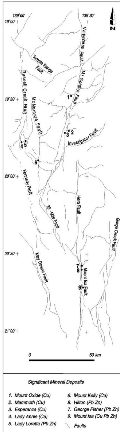
**Figure 2 :** Structural setting of mineral deposits in the central part of the western Mount Isa Block showing the close spatial relationship between base metal mineralisation and faults.
