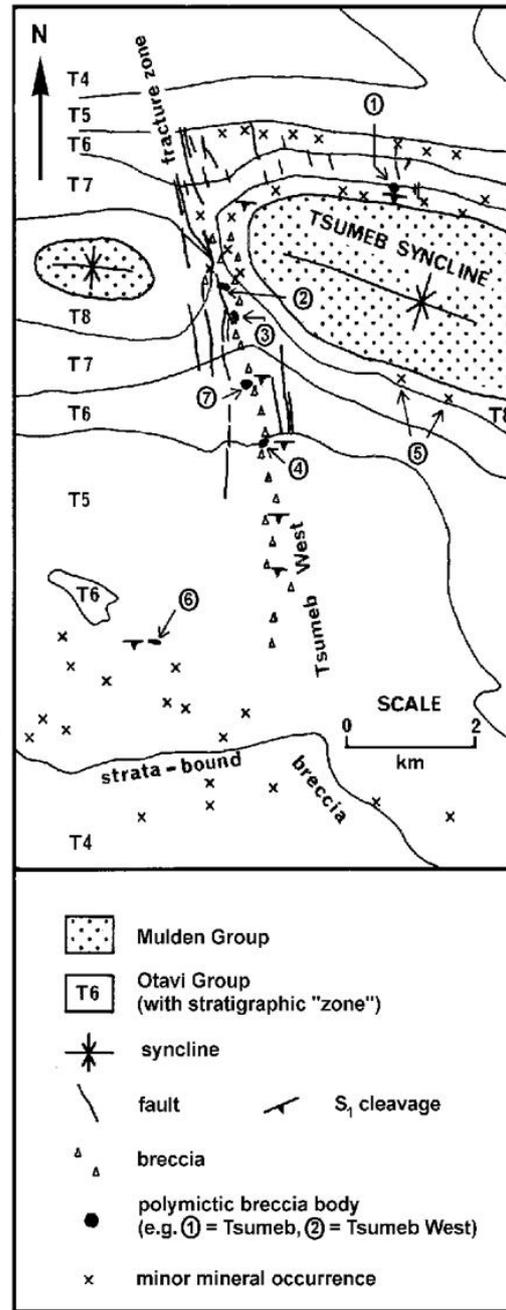
**Figure 9 :** Plan of the Tsumeb orebody and adjacent prospects (Hughes, 1987). Prospects 2, 3, 4 and 7, hosted by polymictic breccia and cavity-filling sandstone, are associated with the Tsumeb West fracture zone. This fracture zone is probably a fault which was karsted prior to deposition of the Mulden Group.
