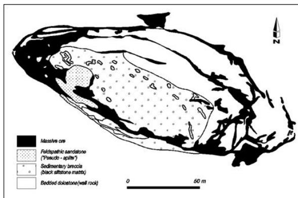
**Figure 5** : Plan view of the Tsumeb orebody at 24 level (simplified from Lombaard *et al.*, 1986). Arcuate, steeply-dipping ring fractures of massive sulphide replace sandstone and dolomite breccia within fractures at the pipe margin. The fractures cut bedded dolomite and rim a pipe-like core of sandstone, black siltstone and dolomite breccia in the southwest part of the pipe. The ring fractures are interpreted to have been more circular in plan prior to folding.
