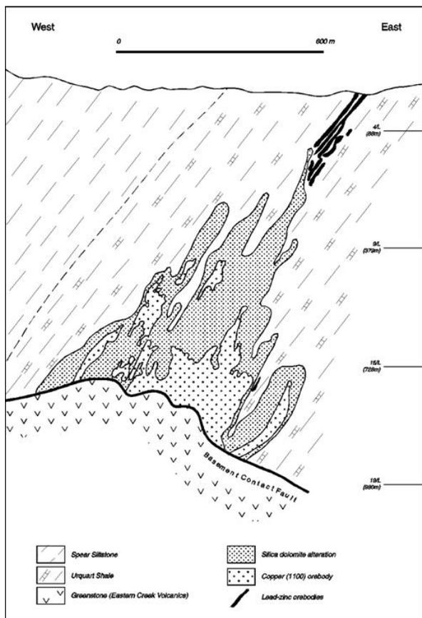
**Figure 3 :** Typical cross section, central mining area, Mount Isa. Copper mineralisation is hosted by pyritic, carbonaceous and dolomitic Urquart Shale above a sub-horizontal fault. Copper mineralisation is associated with intense alteration (silica-dolomite) and cuts and interfingers with lead-zinc mineralisation up-dip.
